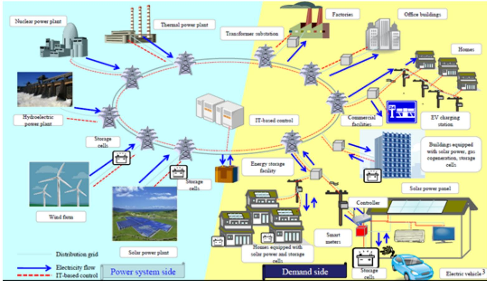
**Smart grid** is the concept of intelligent power network to meet the need of electrical energy by making use of information technology and communication technology in both directions between electricity producers (power system side) and consumers (demand side). The benefits of smart grid technologies are : energy efficiency, flexible power supply, self healing network capability, customer participation and high quality
